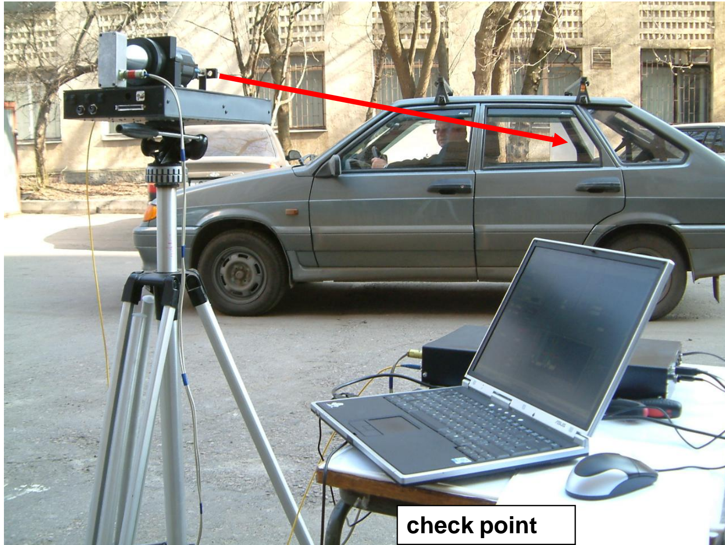
View of field test of NH 3 measurements inside moving vehicle
